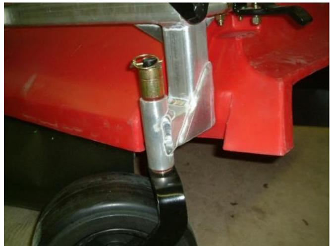
**Figure 4: Castor wheel and boom height spacers**
