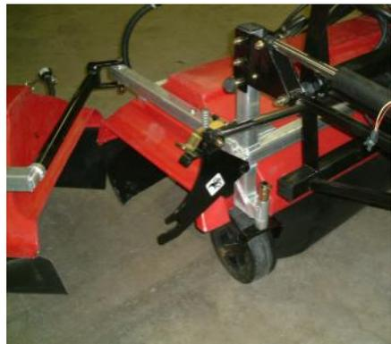
**Figure 14: Extend wing actuator**
