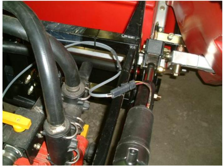
**Figure 26: Slack in wire from frame to actuator**
