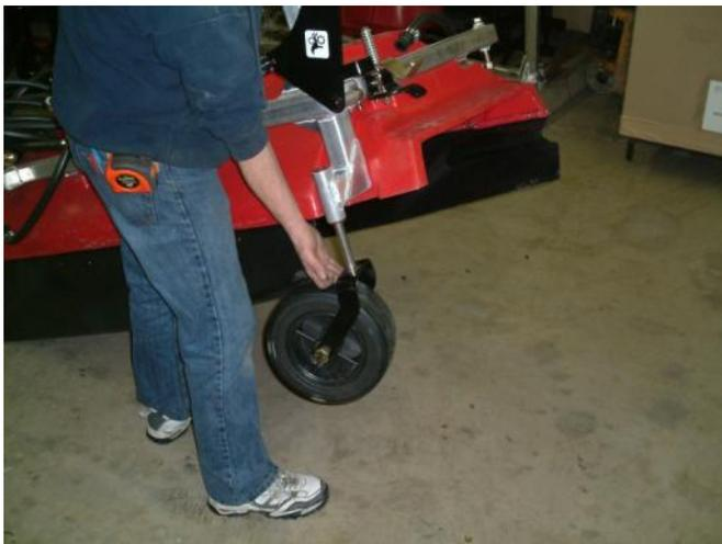
**Figure 3: Inserting castor wheel**
