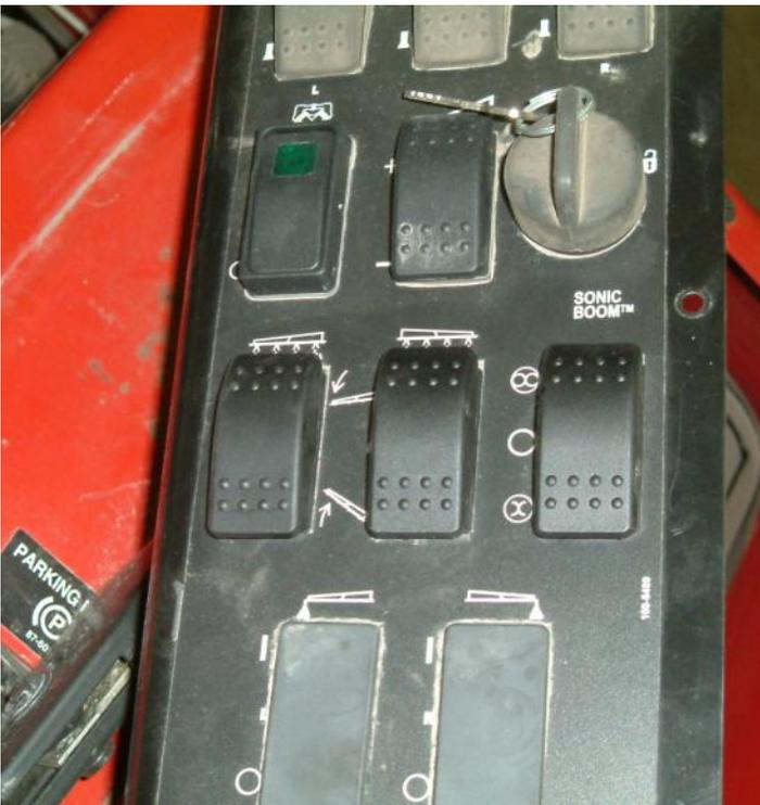
Figure 21: Rocker Switches in Console Panel
