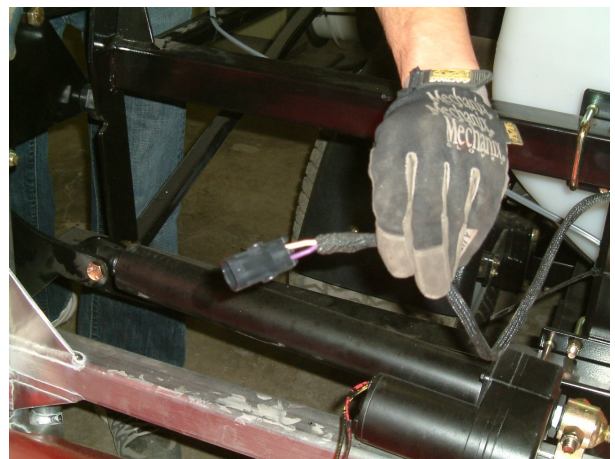
Figure 4: Installed Weather-Pak end
