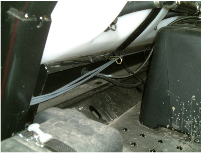
Figure 26: Wire placement along tank
